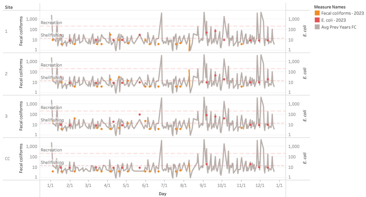
Fig. 14. Fecal coliform (orange) and E. coli (red) densities were lower than Recreational Water Quality Standard (200 cfu/100 ml) but occasionally higher than the Shellfishing Standard (14 cfu/100 ml).
