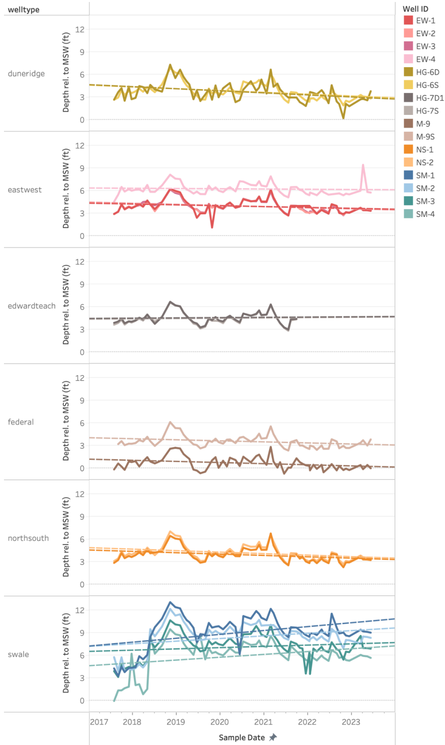
Fig. 3. Depth of groundwater relative to mean sea level (MSL) for each Bald Head Woods well, 2017 - 2023. Higher values represent larger aquifer volume at a particular site through time. Wells HG7D1 and HG7S were removed in 2021 due to development of the lot.
