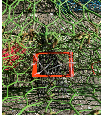
Fig. 35. Terrapin excluder device (TED) on crabpot.
